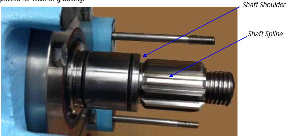
Figure 21 - Shaft Inspection Points
